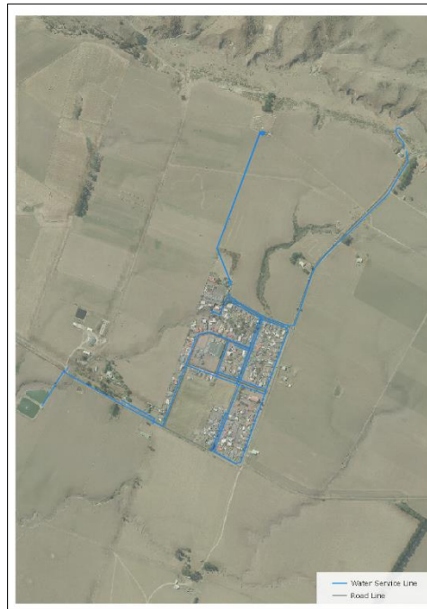
Figure 25: Rātana Water Supply
