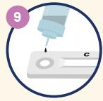
Turn vial upside down and hold sample over sample well. Squeeze vial gently. Allow the required drops according to the kit instructions, to fall into the sample well.
