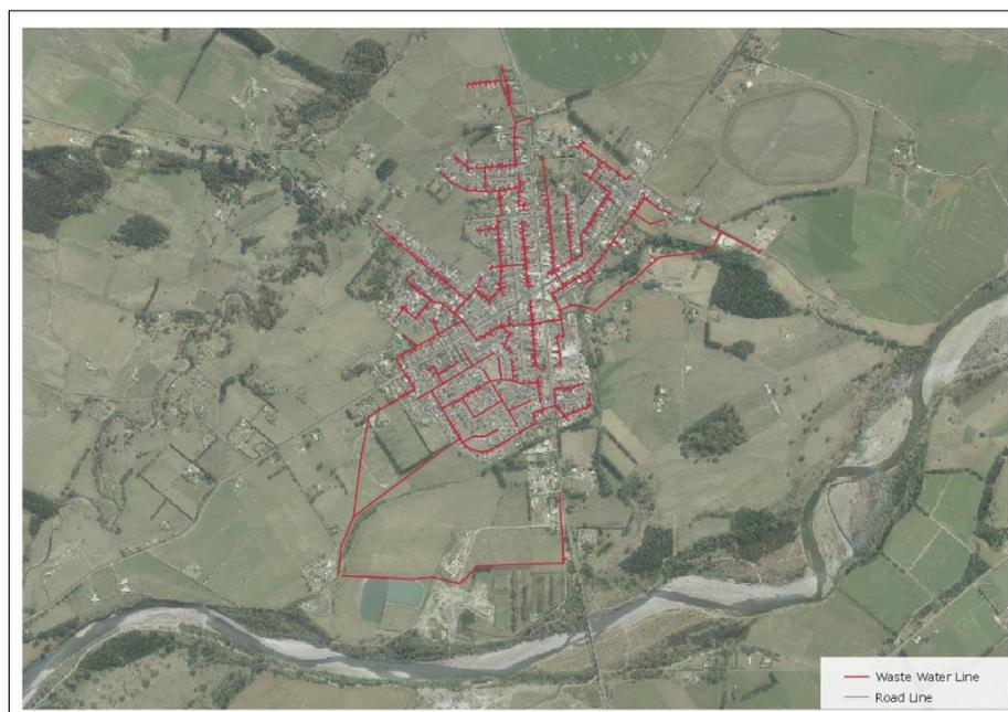
The Bulls wastewater network comprises pipelines ranging from 100 to 375 mm in diameter. The network is relatively young with an age of less than 40 years. The majority pipe material is Asbestos Cement, which has exhibited accelerated deterioration in other communities. However, there is very little industrial waste in the township and the expected remaining life for this material is expected to be longer than elsewhere.
