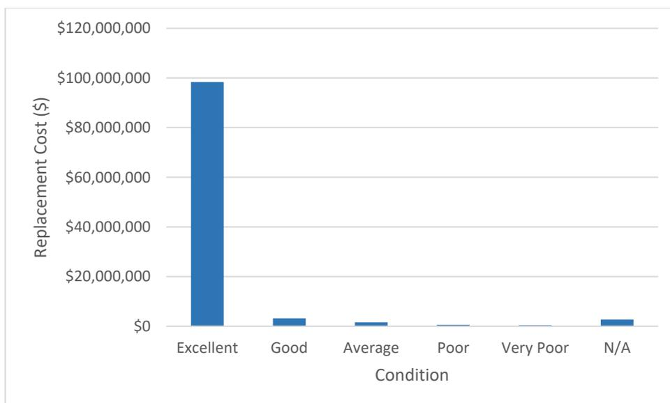
The condition rating of “N/A” is used for assets where no condition information is available. All the assets are recorded on the asset management system, but some recorded assets do not contain any data on condition. Water supply assets shows 7% of recorder assets as having no condition rating data and marked as “N/A”. Improvement of condition information will be completed over the next 3 to 4 years as part of the new asset management strategy.
