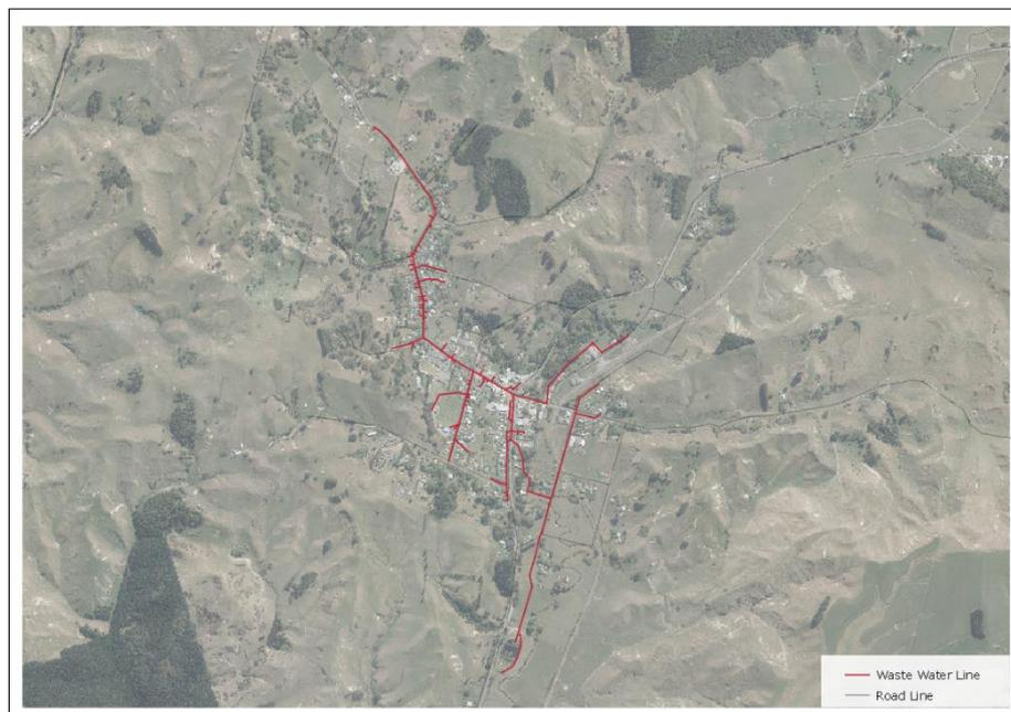
Graphs of pipe age and material for the wastewater system in Hunterville follow. 50% of the reticulation was installed in the 1910s, and is now around 100 years old.
