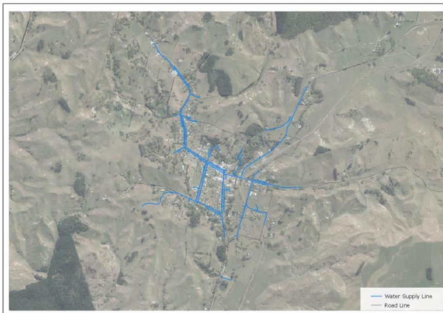
The Hunterville Water Network comprises pressure mains ranging up to 150 mm diameter. The network is relatively new, with no pipes listed as being older than 30 years, and 30% being less than 10 years old.
