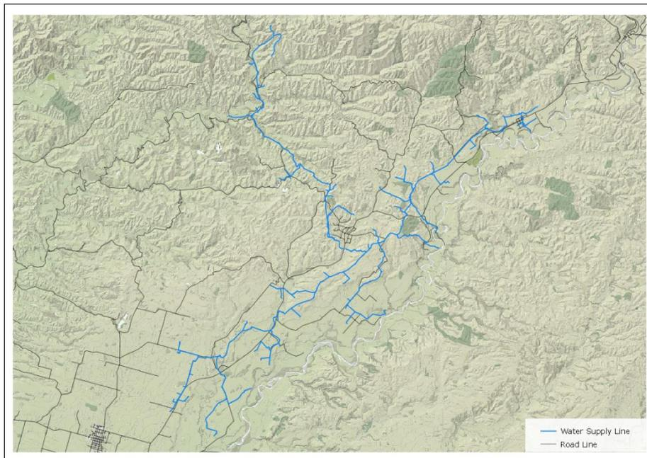
The water network comprises pressure mains ranging up to 150 mm diameter. Nearly the entire scheme was constructed in 1985 from PVC pressure pipe. Some growth of the system occurred in early 2000. Replacement of pipelines has been initiated by mains breaks or land slippage. Extent of replacement has been minimized to only that required to resolve the issue.
