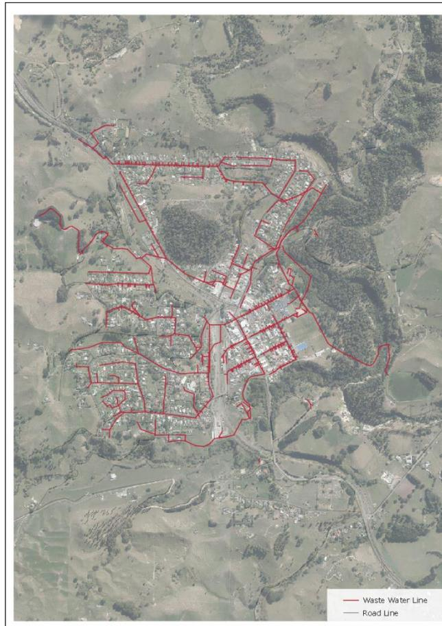
The Taihape wastewater network comprises pipelines ranging from 100 to 375 mm in diameter. Approximately 70% of the network is thought to be glazed earthenware pipes over 90 years old.
