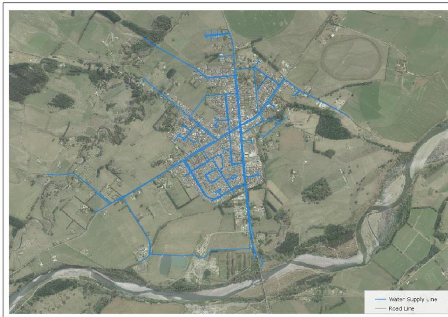
The Bulls water network comprises pressure mains ranging up to 200 mm diameter. Approximately two-thirds of all the pipes are Asbestos Cement pipes laid in the late 1960s and 1970s. This material was superseded in the late 1970s by MDPE and PVC, which now account for 30% of the network. There is a small portion of the network built from copper which is known to be in poor condition.
