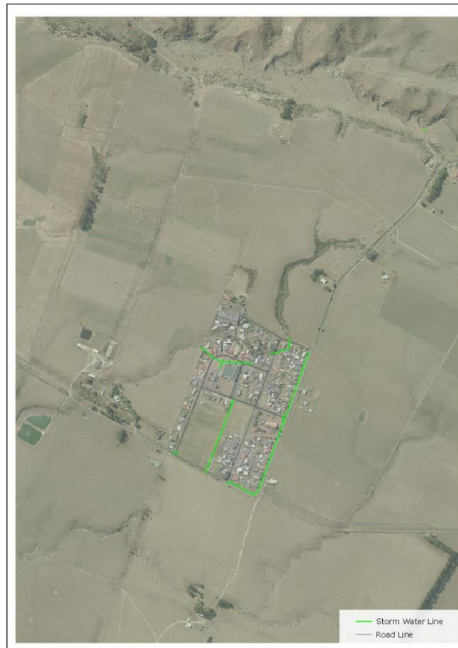
Stormwater pipes in Rātana are either concrete or uPVC. See below.
