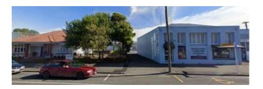
The Marton Library is an earthquake prone building. The WSP seismic assessment dated 3 December 2021 rated the building as 18% of New Building Standard (NBS). It represents a seismic risk to occupants of more than 25 times greater than expected for a new building, indicating a very-high life-safety risk exposure.
