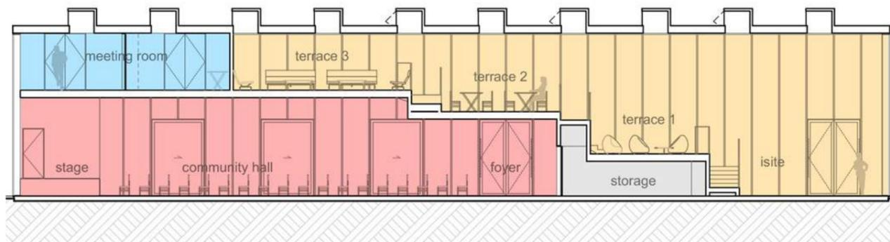
Figure 55: Section through the building showing stepped library terraces with a high stud below for the community hall
