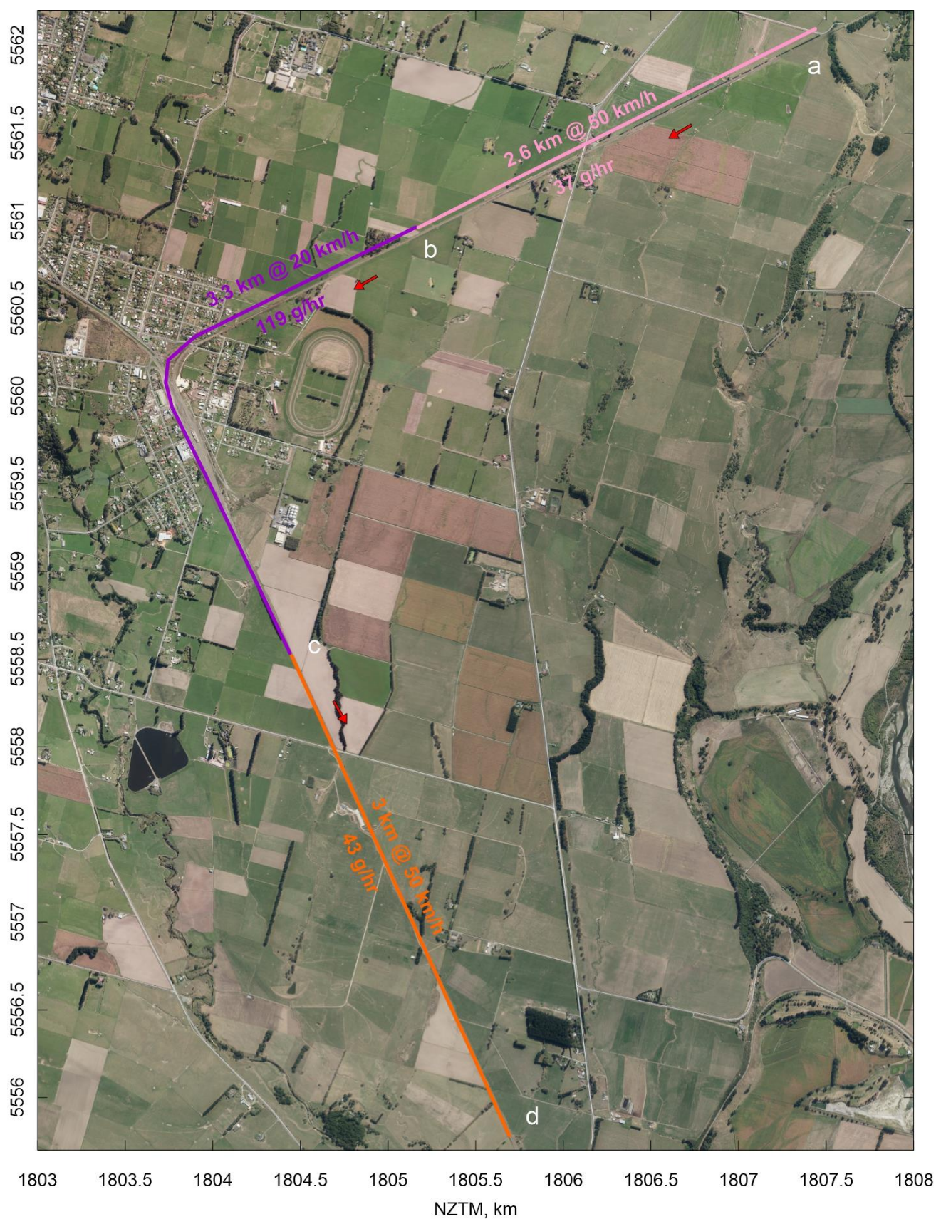
Figure D3: Train speed assumptions and calculated emission rates for trains passing through the new rail siding (baseline scenario).
