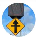
Powered by solar panels, the signs work with sensors on Makirikiri Road sending a signal to the signs on Pukepapa Road when a vehicle is approaching the intersection. The signs will then instruct drivers to slow their speed to 70km/h.
