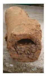
26. It is not adequate to simply put in a drainage system designed for the downside property if it is done in a way that blocks the field tiles. Free flow from the tile system, including adequate identification of the whereabouts of the tile system, and care not to damage the tiles where they enter the downside property, would be required to prevent blockage and potential saturation of the Walsh's property.
