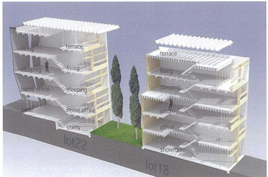
section through both buildings on two lots to show the various functions on each level
