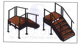
Steps to be made from aluminium in two pieces: the stairs and the landing (can be used as required)
